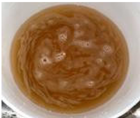
Figure 5. Unstable foam generation observed in the presence of organics, excluding saponin, following vigorous shaking
