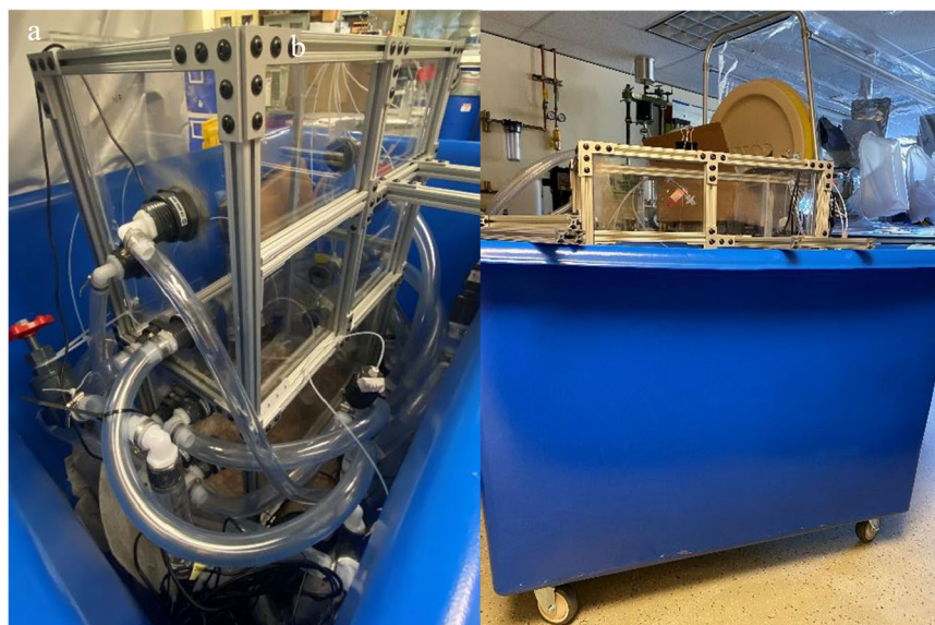
Figure 16. Experimental lake simulator flow cell showing (a) polycarbonate sheets with aluminum frame to provide structural rigidity and (b) secondary plastic containment
